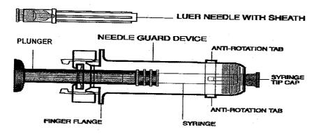
NOTE: Please use the enclosed needle for administration. If a different needle is chosen, it should fit securely on the syringe and be no longer than 1 inch to ensure proper functioning of the needle guard device. Two detachable labels are provided which can be removed after the needle is guarded.
